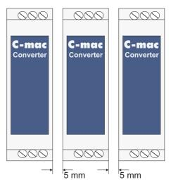
Please note, that the units must be installed with minimum 5 mm gap, because of the internal heat generation.
